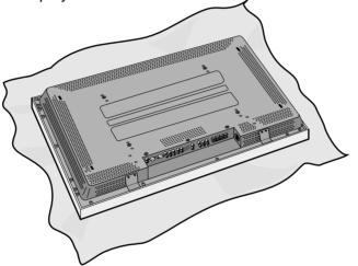
•Take the speakers with fixed brackets to the back of the plasma display. Place the hooks onto the fixed brackets to the squared holes in the back of the plasma display.
